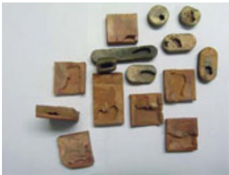
Over compressing certain rubber products destroys the cells within the rubber.
