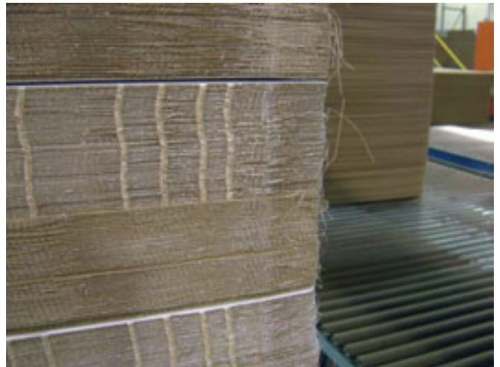
Flatbed cutting dies which cut onto steel plates give us warning signs that things are going south in the way of “angel hair” clinging to the units.
