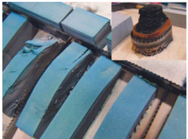
Damaged rubber that has been worn down or stacked double up
