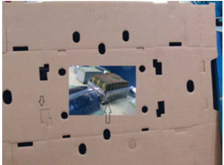
A small gap of only 1/16" (1.5mm) on a knife such as a small vent hole cutout is trouble.
